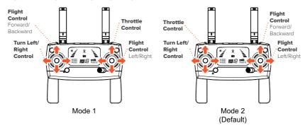
In **MODE 1** the right control stick controls the throttle. In **MODE 2** the left control stick controls the throttle. The factory settings in the remote control are set to **MODE 2** (Default).
